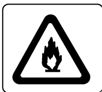
WARNING - Flammable liquid.
