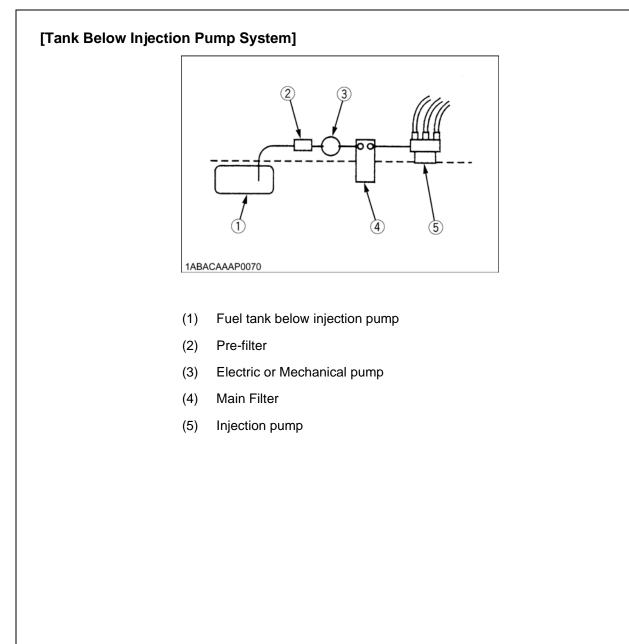
Checking the Fuel Pipes
