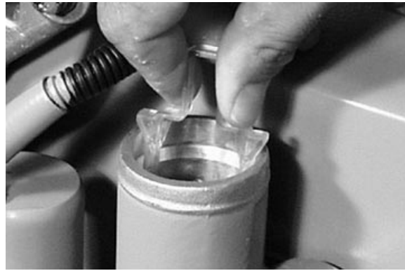
Removing Thermostat from Housing
