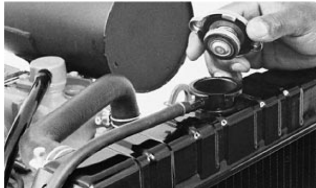
Check Coolant Level in Radiator
