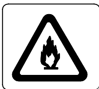
WARNING - Flammable liquid.
