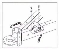
Figure 2 Safety Chain Attachment
