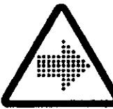
WARNING – Air/gas flow or Air discharge.
