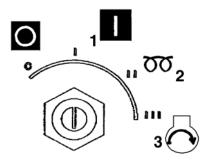
All normal starting functions are incorporated in the key operated switch.
