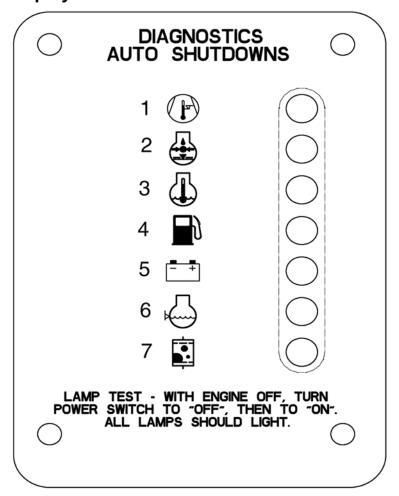
The diagnostic display panel is arranged as shown above. A description of each diagnostic indicator is as follows.
