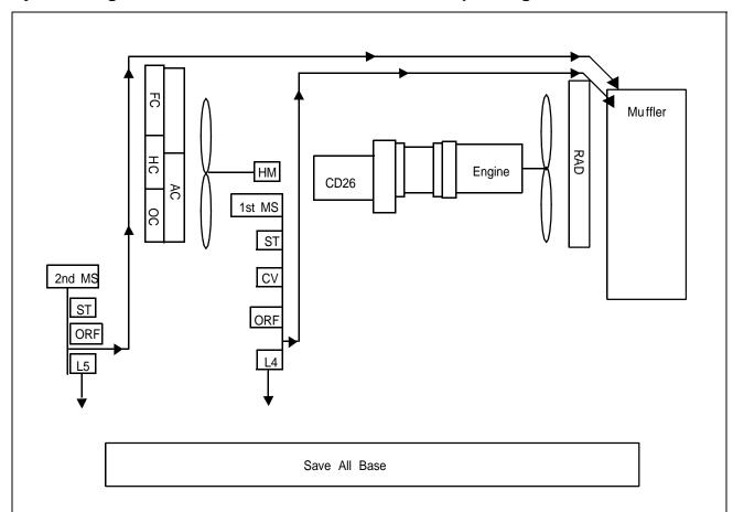
Figure - 7 Condensate Flow Schematic
