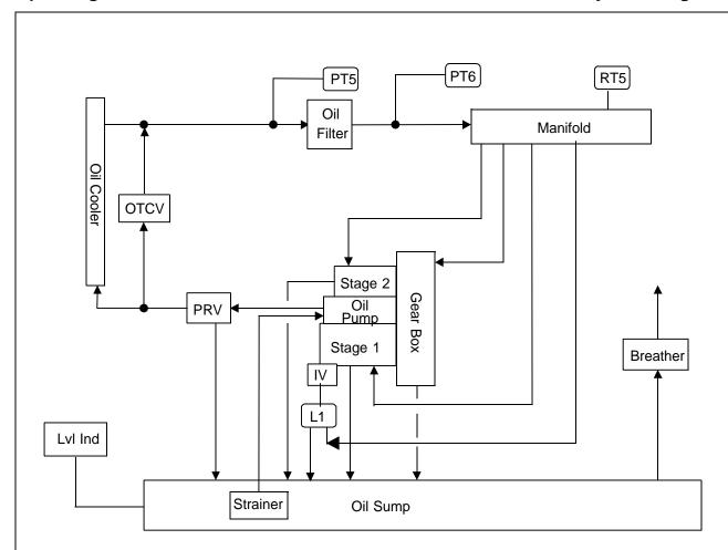
Figure 2: Lube Oil System Schematic
