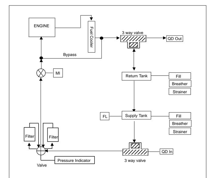
Figure 4: Fuel System Schematic
