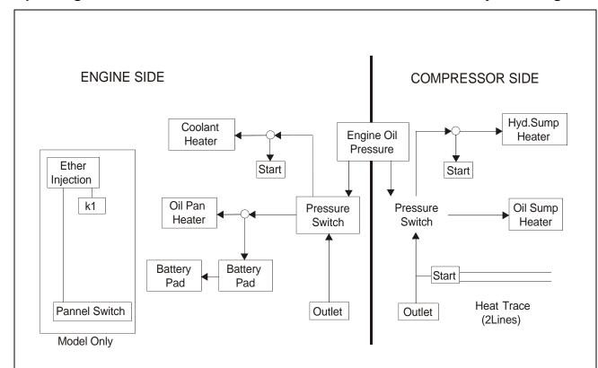
Figure 6 : AC Cold Start System Schematic
