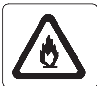
WARNING - Flammable liquid.
