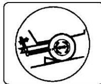
When parking use prop stand, handbrake and wheel chocks.
