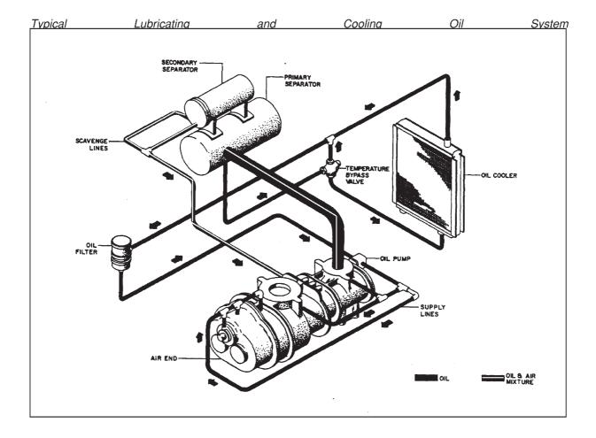
Relatively cool lubricating oil is admitted under pressure to the compressor bearings and is also injected in metered amounts, directly to the rotor chamber. All of the oil thus introduced mixes with, and passes on with the air being compressed, thus removing the heat of compression to a large degree. On its way to the final discharge connection, the air passes through a receiver/separator. A scavenger line returns any remaining separated oil back to the inlet of the compressor.
