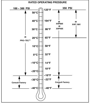
Preferred Ingersoll-Rand Fluids - Use of these fluids with original I-R filters can extend airend warranty. Refer to operator's manual warranty section for details or contact your I-R representative.
