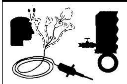
Air pressure can remain trapped in air supply line which can result in serious injury or death.
