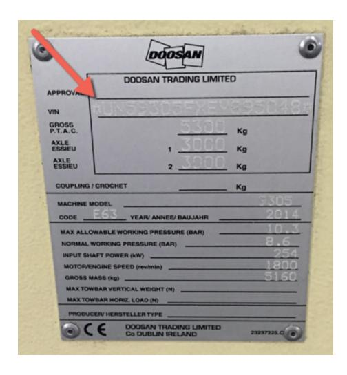
Compressors produced in the EU will show this dataplate on the outside of the unit.
