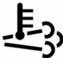
Engine emissions system temperature may be high.
