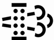
Operational status of the engine emission filter.
