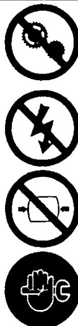
**WARNING** – Do not undertake any maintenance on this machine until the electrical supply is disconnected and the air pressure is totally relieved.
