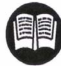
Read the Operation and Maintenance manual before operation or maintenance of this machine is undertaken
