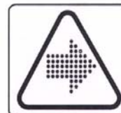
Air/gas flow or Air discharge.
