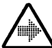
**WARNING** – Air/gas flow or Air discharge.
