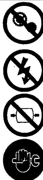
**WARNING** – Do not undertake any maintenance on this machine until the electrical supply is disconnected and the air pressure is totally relieved.
