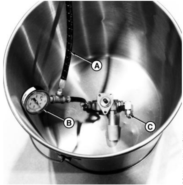
Fuel Supply Pump Leak Test
