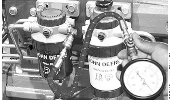
In-Line Supply Pump Pressure
