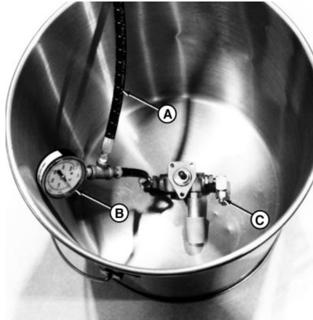
Fuel Supply Pump Leak Test
