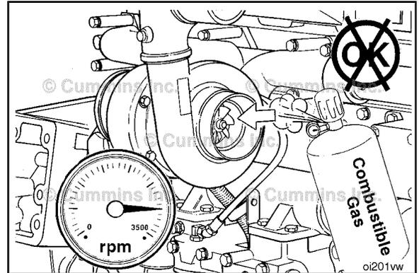
Cummins recommends the installation of an air intake shutoff device or a similar safety device to minimize the risk of overspeeding where an engine, due to the vehicle, vessel or equipment being operated in a combustible environment, such as due to a fuel spill or gas leak.
