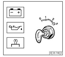
• Turn key anticlockwise (to position 0) and remove. Pilot lights will go out.
