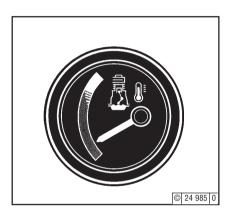
Engine temperature gauge pointer should remain in green sector most of time. It should rarely enter yellow-green sector. If pointer enters orange sector, engine is overheating. Turn off and establish cause from Fault Table (see 7.1).
