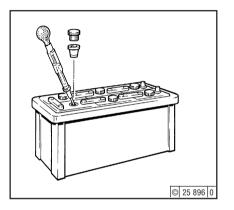
Measure electrolyte density of individual cells with commercial hydrometer.
