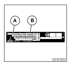
The model **A**, the engine serial number **B** and the performance data are stamped on the rating plate. The model and engine serial number must be given when ordering parts.
