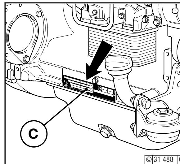
The nameplate **C** is attached to the crankcase.
