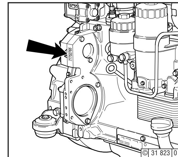
The engine serial No. is stamped on the crankcase and also on nameplate..
