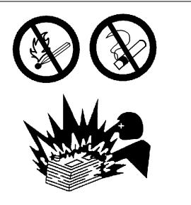
Gases from a battery can explode. Keep any open flames or sparks away from the top of a battery. Do not smoke in battery charging areas.
