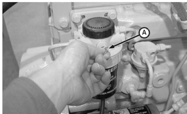
Final Fuel Filter Bleed Vent Screw
