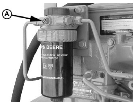
Final Fuel Filter Bleed Vent Screw
