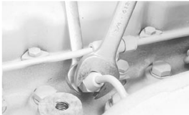
Bleeding Fuel System at Injection Nozzle
