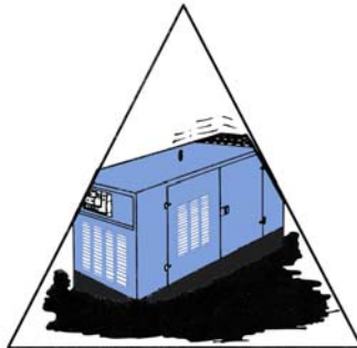
Ground too uneven or soft. Set incorrectly positioned
