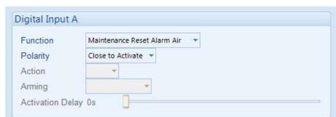
**Example 3:** Screen capture from DSE Configuration Suite Software showing the Maintenance Alarm Reset 'button' in the DSE Configuration Suite SCADA | MAINTENANCE section.
