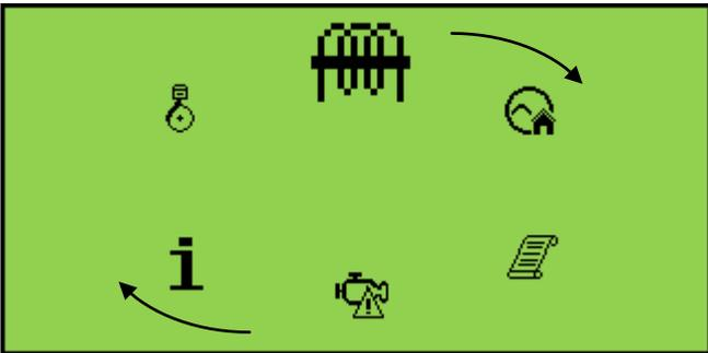
Once the desired icon is at the top, press the *Auto Mode*
