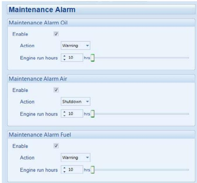
When activated, the maintenance alarm can be either a *Warning* (set continues to run) or *Shutdown* (running the set is not possible).
