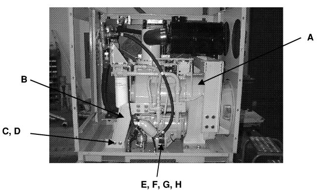
**ITEM PART NUMBER DESCRIPTION** XHP825CMH @1800 rpm / XHP900CMH @ 2100 rpm Α 35086354 XHP650CMH/XHP750CMH ((2100 rpm) 35086347 35096205 XHP750CMH (1850 rpm) XHP825CMH (2100 rpm) 35089879 35097468 XHP900CMH (1800 rpm) CompressorAssy (see dwg 36735967 for parts breakdown) В 43212026 Support RH Support LH (opposite side) 43212018 C 35252568 **Bolt (4)** D 35252618 Nut (4) Ε **Check Valve** 36843720 F 95225116 Gasket (2) G 35376094 **Bolt (8)** Н 11A5G8 Washer (8)
