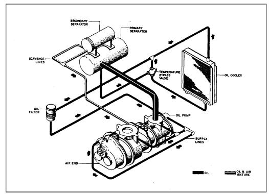
Relatively cool lubricating oil is admitted under pressure to the compressor bearings and is also injected in metered amounts, directly to the rotor chamber. All of the oil thus introduced mixes with, and passes on with the air being compressed, thus removing the heat of compression to a large degree. On its way to the final discharge connection, the air passes through a receiver/separator. A scavenger line returns any remaining separated oil back to the inlet of the compressor.
