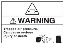
Close service valve and operate tool to vent trapped air before performing any service
