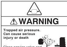
Close service valve and operate tool to vent trapped air before performing any service
