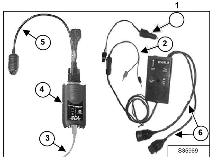
Select and configure the appropriate cables and adapters for the Level of ECU (Engine Control Unit) to be programmed and the power source to be used.
