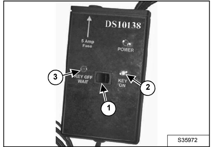
Switch the Main Test Box switch (Item 1) to the "KEY ON" position. The "KEY ON" indicator light (Item 2) [Figure 3] should be ON.
