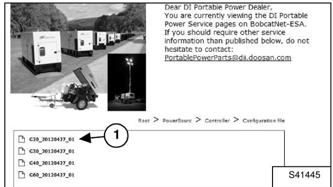
Select the configuration file (Item 1) [Figure 11] corresponding to the generator model you are updating and click to save the files on your computer:
