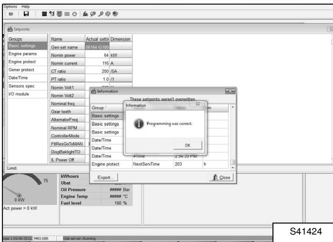
When the screen [Figure 28] is displayed, the programming is completed.
