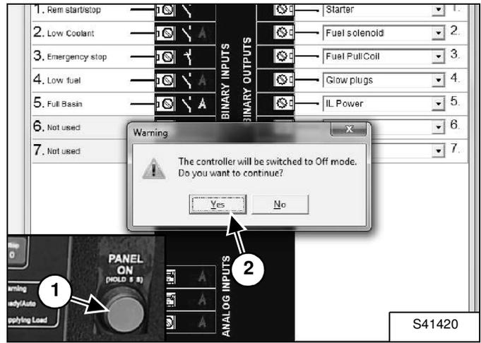
**NOTE:** The controller will be switched off during the programming [Figure 25]. Therefore the controller power hold will be released.
