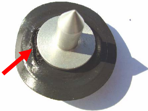
Figure 1 Failed pressure regulator membrane
