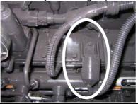
9 Combined Intake Temperature and Pressure Sensor
