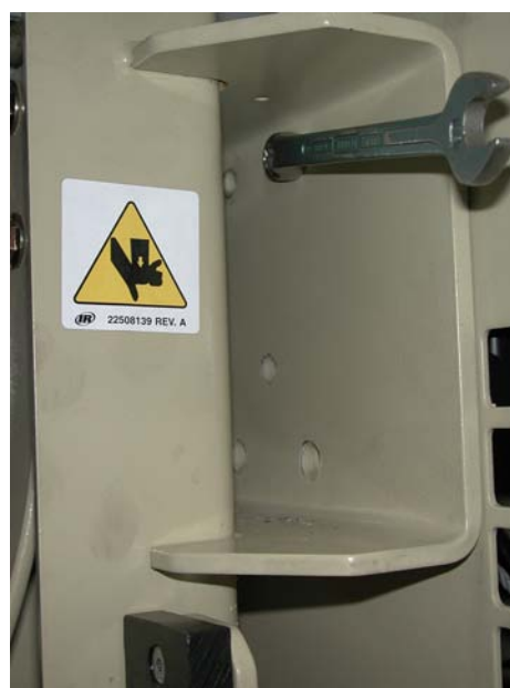
Dismantle winch (5X) with spanner 13mm & 15 mm
