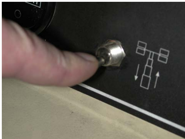
Push the "lower mast" button so that the cable becomes slack on the winch. \pm 0.5 meter
