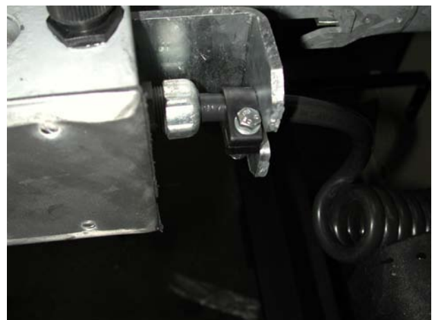
Place a cable clamp on each side of the support. Install first the rubber protection on the cable!
