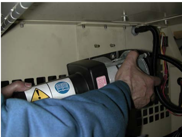
Reinstall the winch
