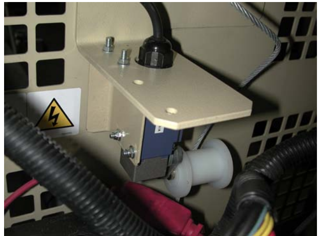
Install the tensioner switch
