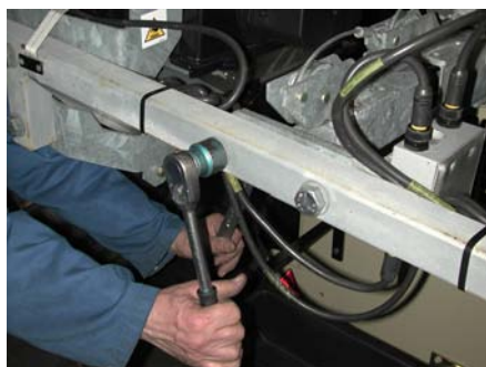
Remove bar with spanner 30mm (2X) and remove junction box support
