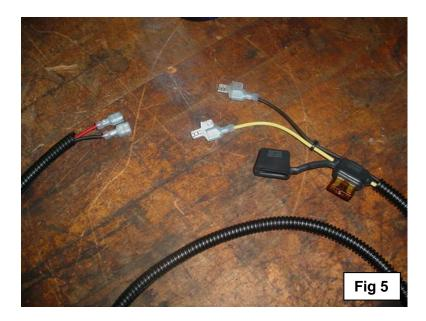
Step 6: Connect the leads of the harness to the heater connections (polarity doesn't matter). Then run the wiring harness along the trailer lighting harness in the lower frame putting a zip/wire tie about every foot to secure it from moving around till the harness reaches the hour meter on the control panel Fig 6.
