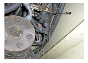
New improved coils are now available for the press-to-drive system on loader backhoes. The new coils are rated to operate at a higher voltage and temperature to provide longer service life. Parts are now available to upgrade earlier loader backhoes with the serial numbers listed above.
