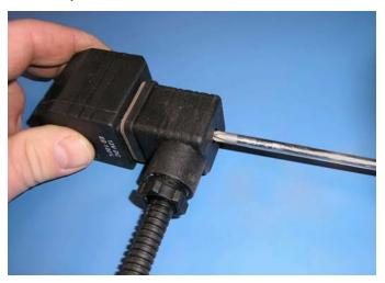
Connect the adapter harness to the new coil. Tighten the screw.
