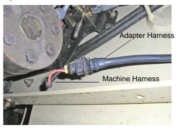
Connect the adapter harness to the machine harness.
