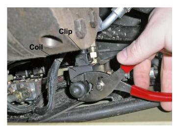
Depress the clip on the wire harness connector, disconnect the wire harness from the coil. Use pliers to loosen the nut, remove the coil from the machine.
