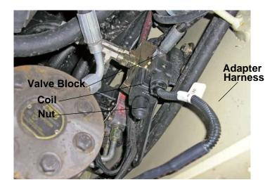
Install the new coil onto the valve block using the original nut. Use pliers to gently tighten the nut until snug.
