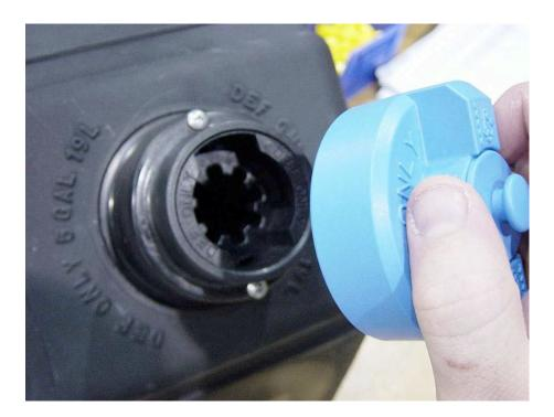
8) Wipe down the fill port adapter with a damp cloth before replacement of the cap. Take the cap and replace with the grooves on the cap fitting into the notches on the fill port adapter.
