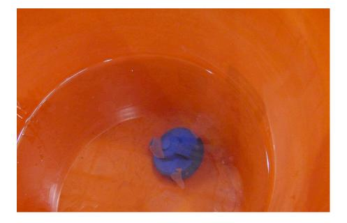
5) After soaking, grip the cap and shake vigorously while underwater to break up and loose and/or remaining DEF within the cap assembly.
