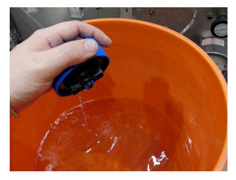
7) Blow off cap to remove any retained water, to prevent freezing when operating in colder climates.
