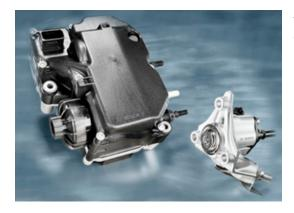
The Bosch pump will deliver DEF fluid to the dosing unit fitted on the Decomposition Tube (DRT) between the DOC and SCR.
