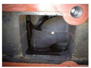
The inside of the chamber is clean and about 99% of the corrosion/impurities was removed.
