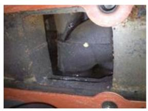
Approximately 90% of the cleaning substance was removed, but a small amount of cleaning substance remains ⇒ Additional Rust Removal Required.
