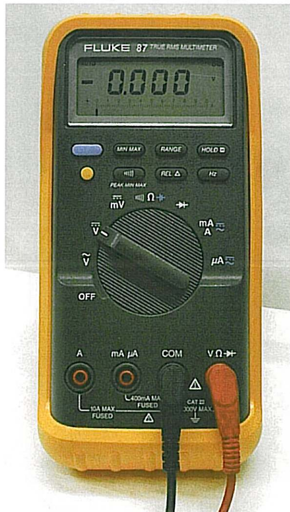
Fluke 87 Configured For Frequency
