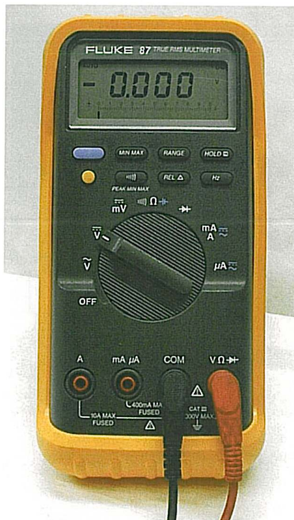
Fluke 87 Configured For Duty Cycle
