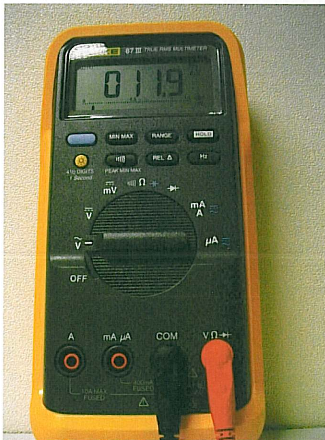
Fluke 87 Configured For AC Volts
