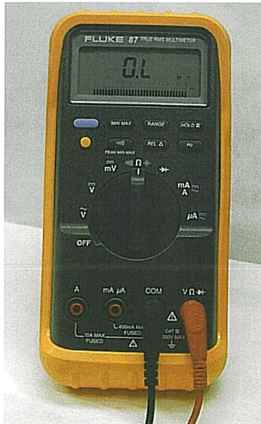
Fluke 87 Configured For Resistance
