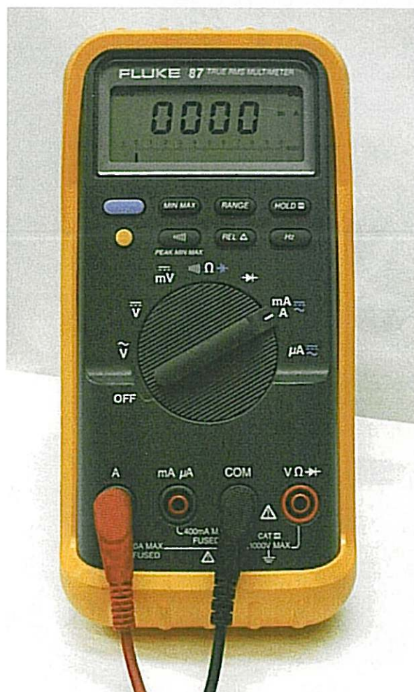
Fluke 87 Configured For Amps
