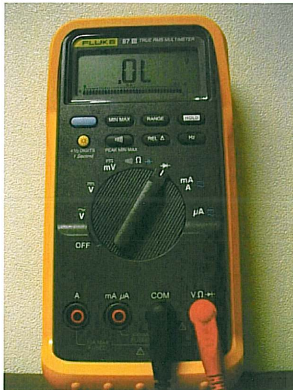
Fluke 87 Configured For Diode Test
