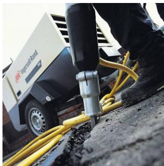
Asphalt work, 7/51 powering a medium duty Paving Breaker
