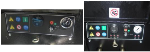
Enhanced control panel on 7/26E & 7/31E
